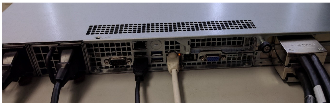
Gen3 Sample Adapters Installed on a SANBlaze VLUN Host System
