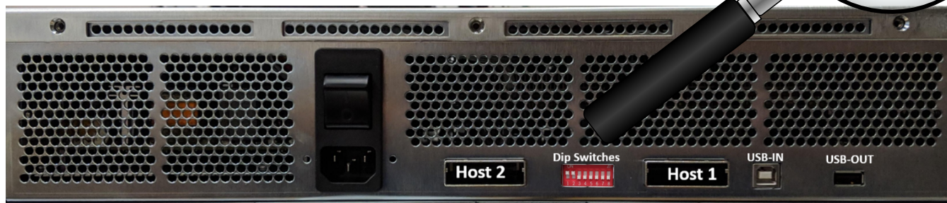
Connect the Gen3 Host (see Step 2) to the SBExpress-RM NVMe Test System (shown here)
